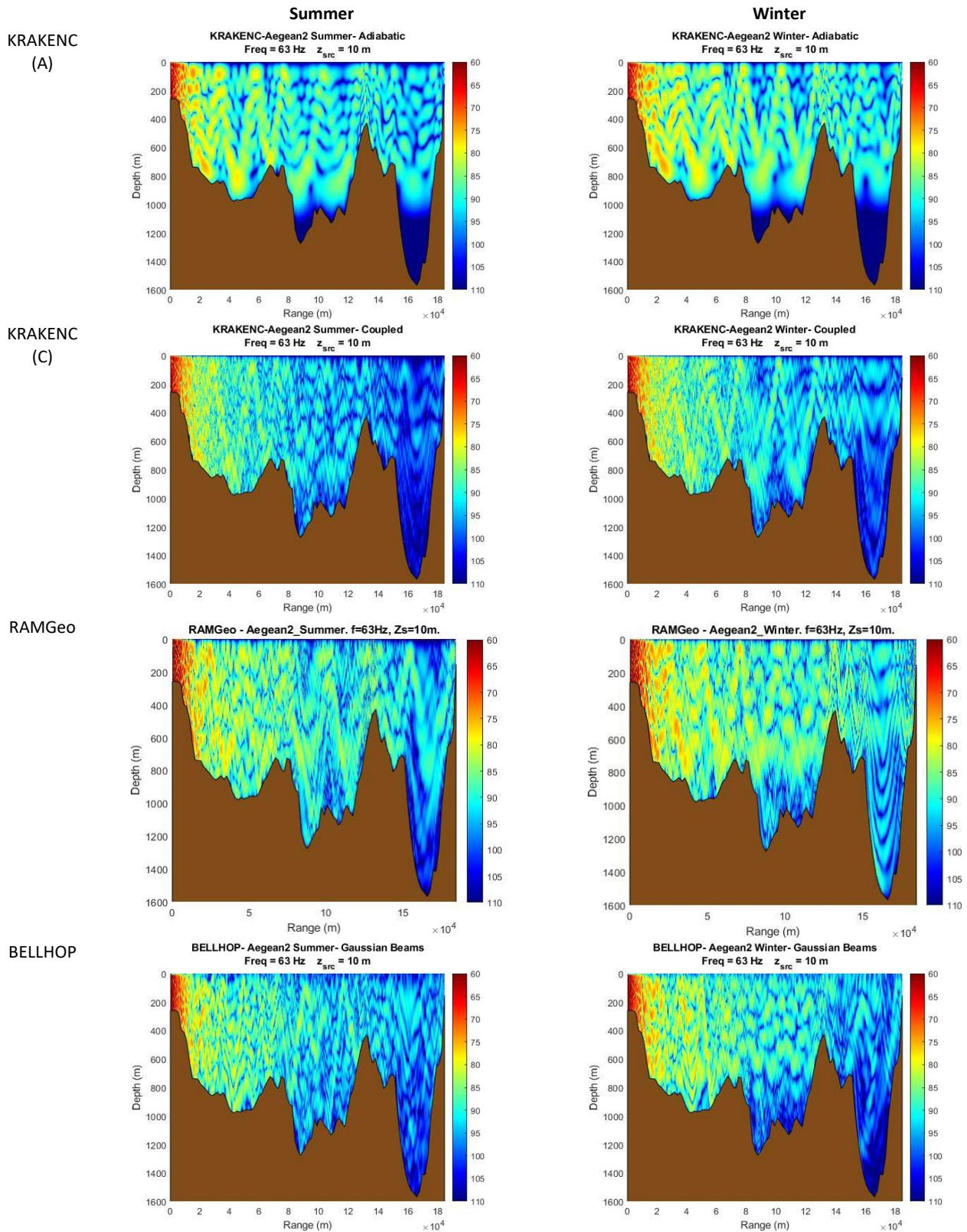
Figure 23. Acoustic propagation models outputs for summer (left column) and winter (right column) profiles and the four considered models (rows) for the Aegean Sea II test site (Area III) at 63 Hz.
