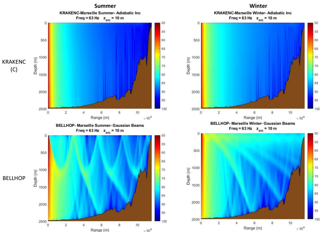
Figure 14. Acoustic propagation models (incoherent mode) outputs for summer (left column) and winter (right column) profiles and two models (KRAKENC Adiabatic and BELLHOP) for the Marseille test site (Area I) at 63 Hz.
