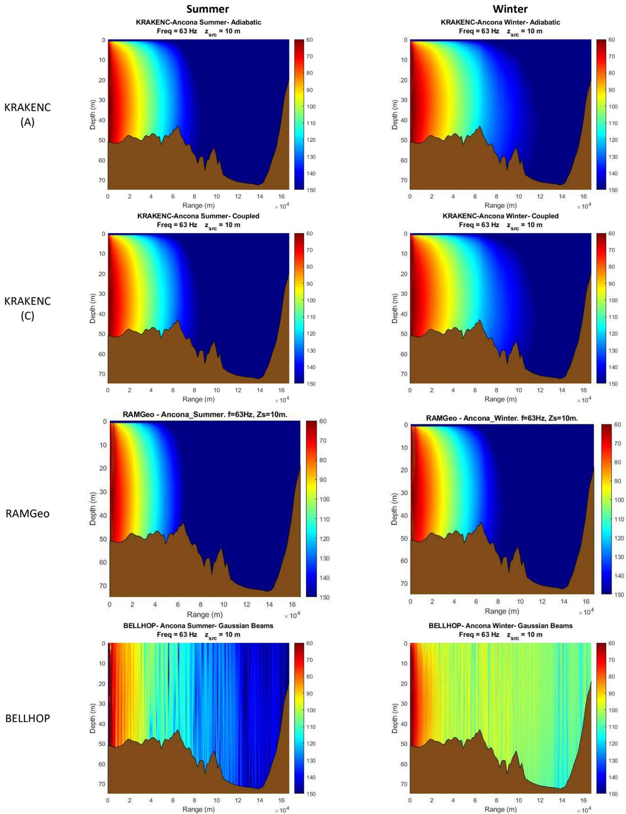
Figure 25. Acoustic propagation models outputs for summer (left column) and winter (right column) profiles and the four considered models (rows) for the Ancona test site (Area IV) at 63 Hz.
