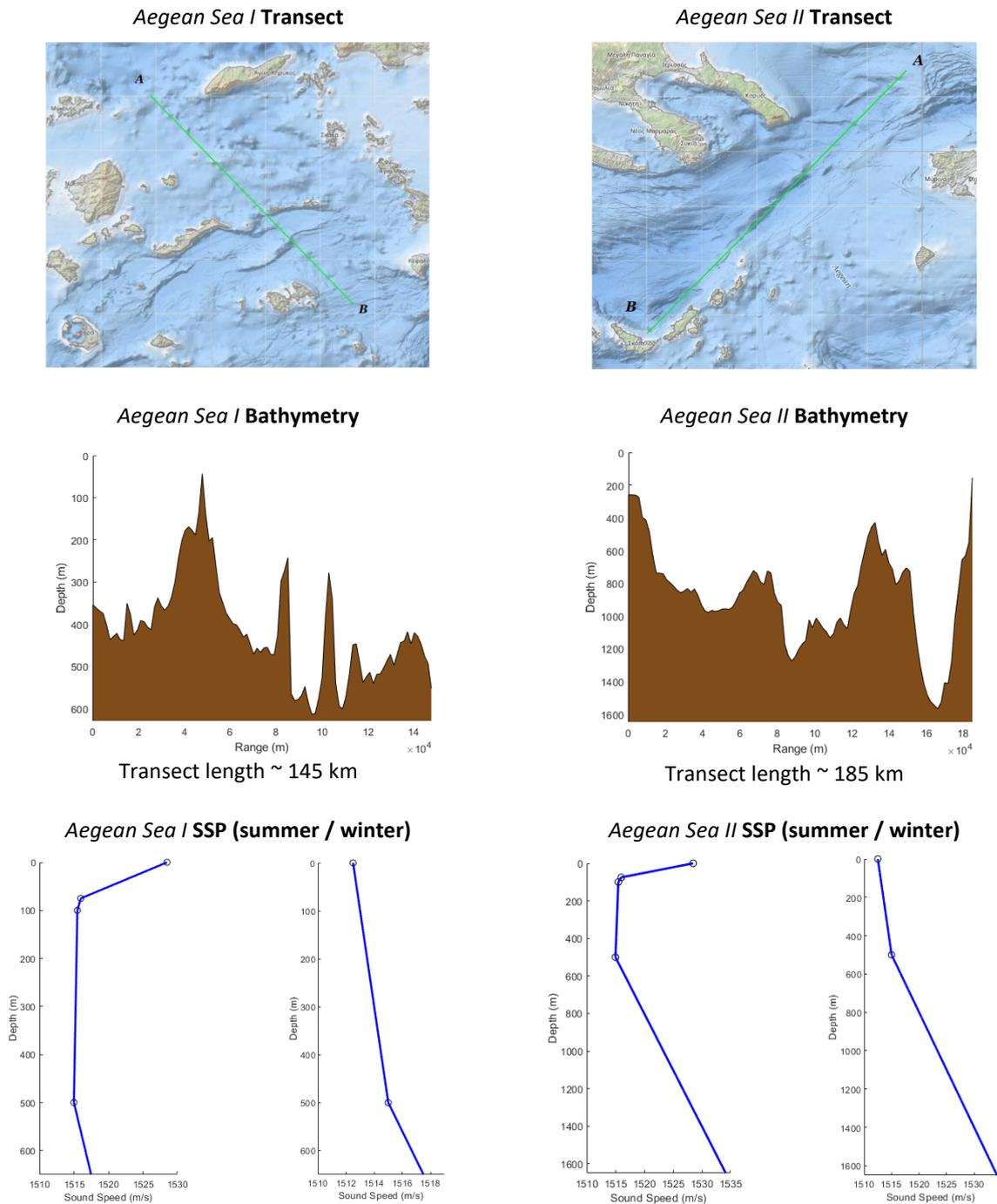
Figure 20. Sites with transects, bathymetric profiles and SSPs for Area III. Propagation transects, the bathymetric profiles and SSPs for Aegean Sea I (left column) and Aegean Sea II (right column).
