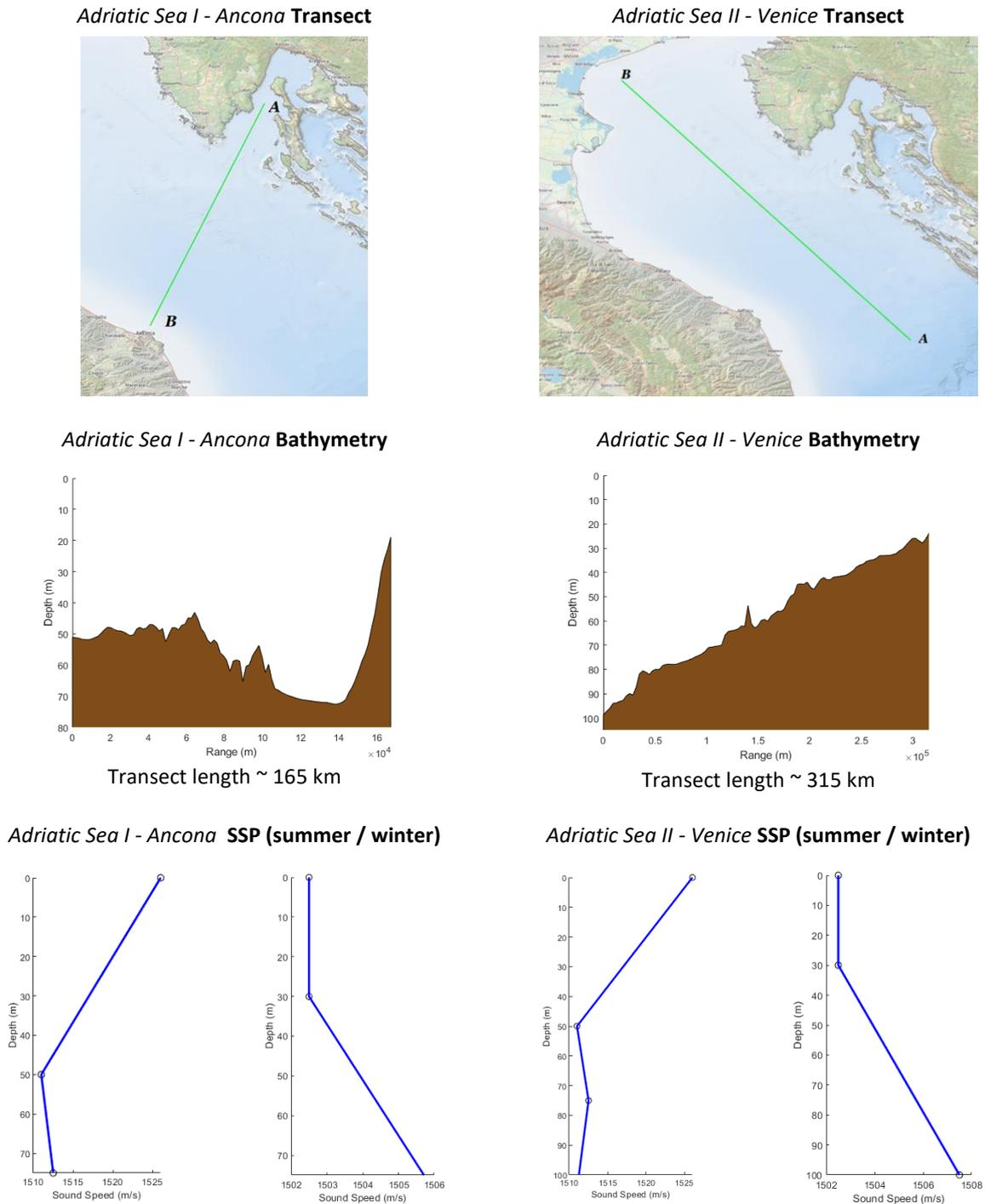
Figure 24. Sites with transects, bathymetric profiles and SSPs for Area IV. Propagation transects, the bathymetric profiles and SSPs for ‘Ancona’ (left column) and ‘Venice’ (right column) test sites.
