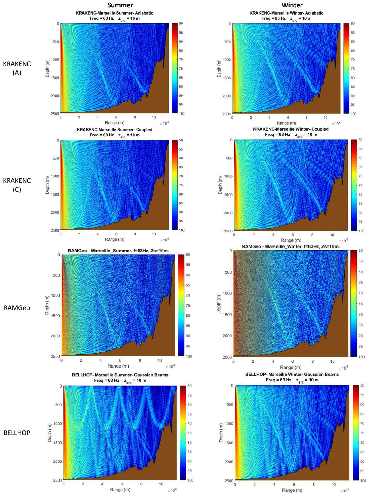
Figure 12. Acoustic propagation models outputs for summer (left column) and winter (right column) profiles and the four considered models (rows) for the Marseille test site (Area I) at 63 Hz.
