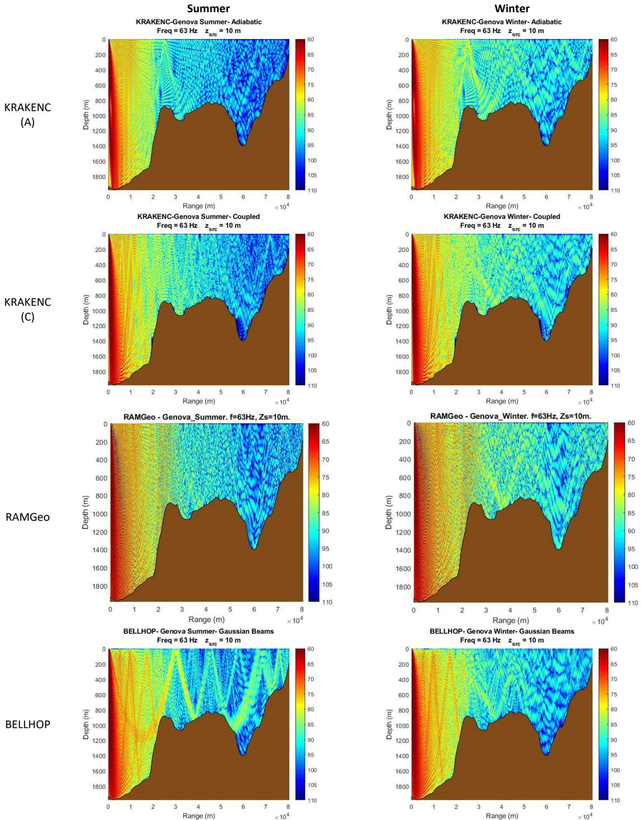
Figure 16. Acoustic propagation models outputs for summer (left column) and winter (right column) profiles and the four considered models (rows) for the Genova test site (Area I) at 63 Hz.
