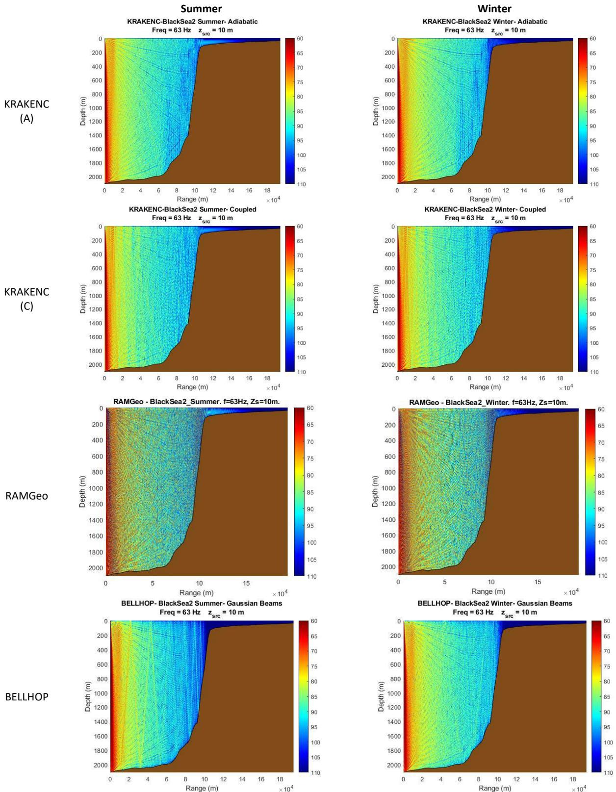
Figure 10. Acoustic propagation models outputs for summer (left column) and winter (right column) profiles and the four considered models (rows) for the ‘Constanza II’ test site (Area V) at 63 Hz.
