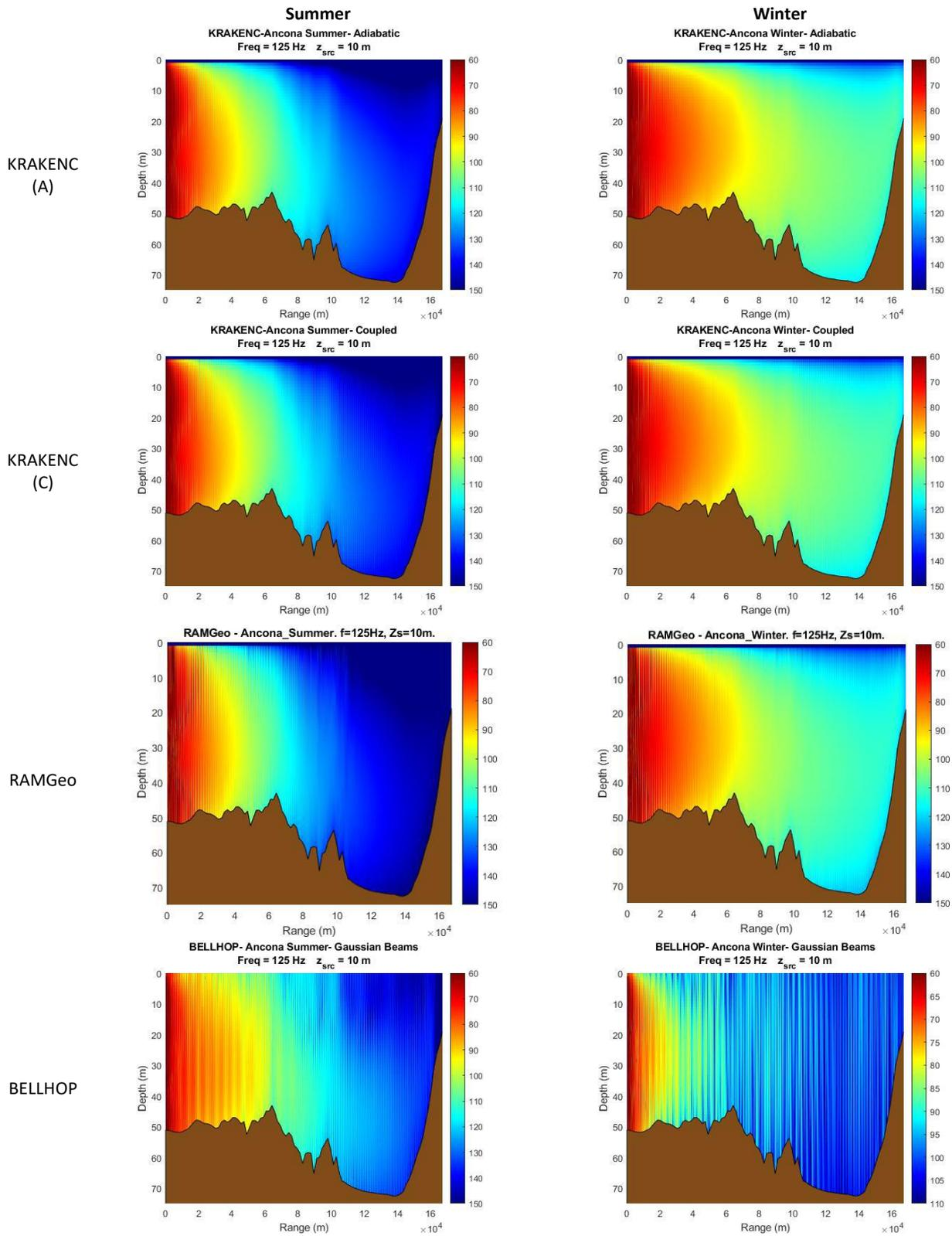
Figure 26. Acoustic propagation models outputs for summer (left column) and winter (right column) profiles and the four considered models (rows) for the Ancona test site (Area IV) at 125 Hz.
