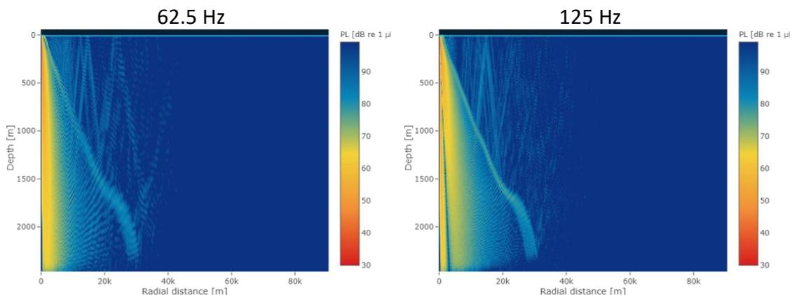
Figure 39. Propagation losses for the Marseille environment (Area I) from the URN tool using the BELLHOP model.
