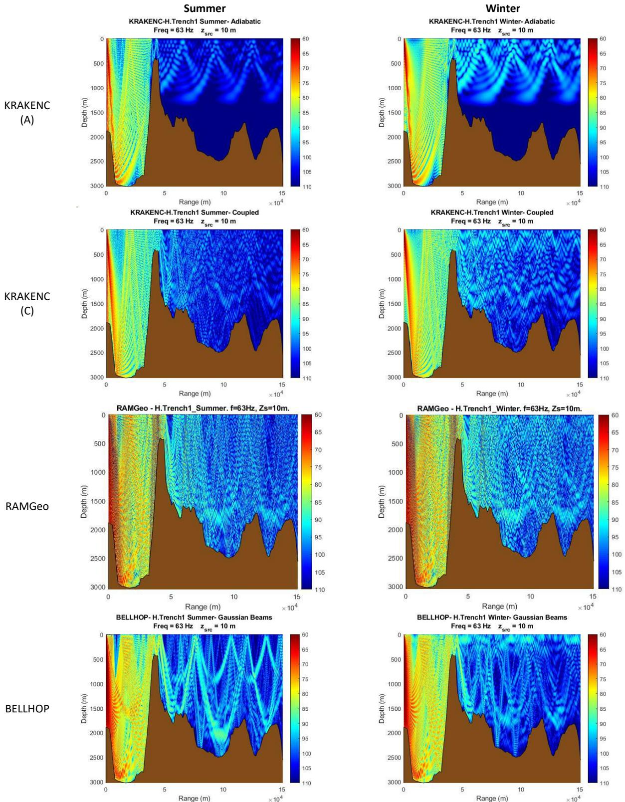
Figure 18. Acoustic propagation models outputs for summer (left column) and winter (right column) profiles and the four considered models (rows) for the Hellenic Trench test site (Area II) at 63 Hz.
