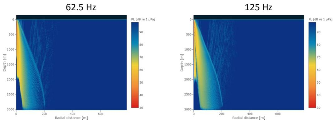
Figure 41. Propagation losses for the Hellenic Trench environment (Area II) from the URN tool using the BELLHOP model.
