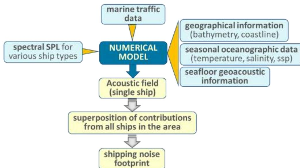
Figure 1. The process of numerical modelling for estimating the shipping noise footprint of a marine area (slightly modified from Prospathopoulos et al., 2019).
