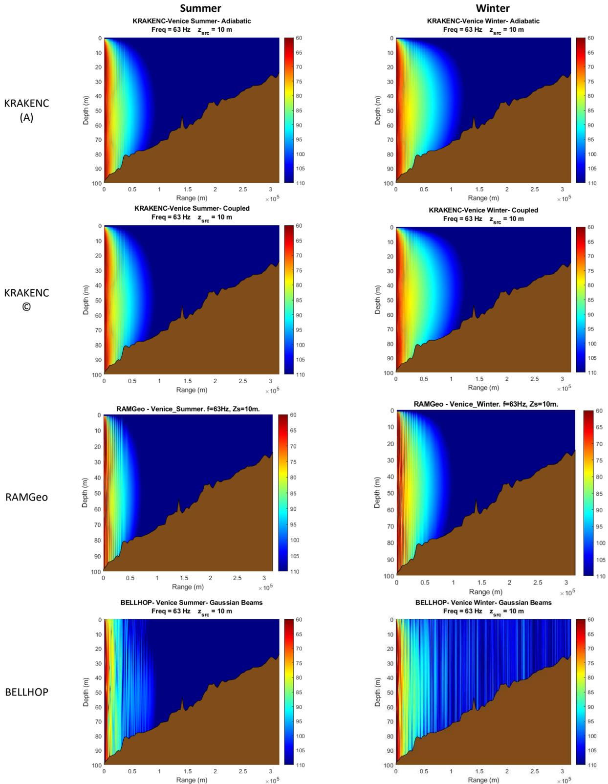
Figure 27. Acoustic propagation models outputs for summer (left column) and winter (right column) profiles and the four considered models (rows) for the Venice test site (Area IV) at 63 Hz.
