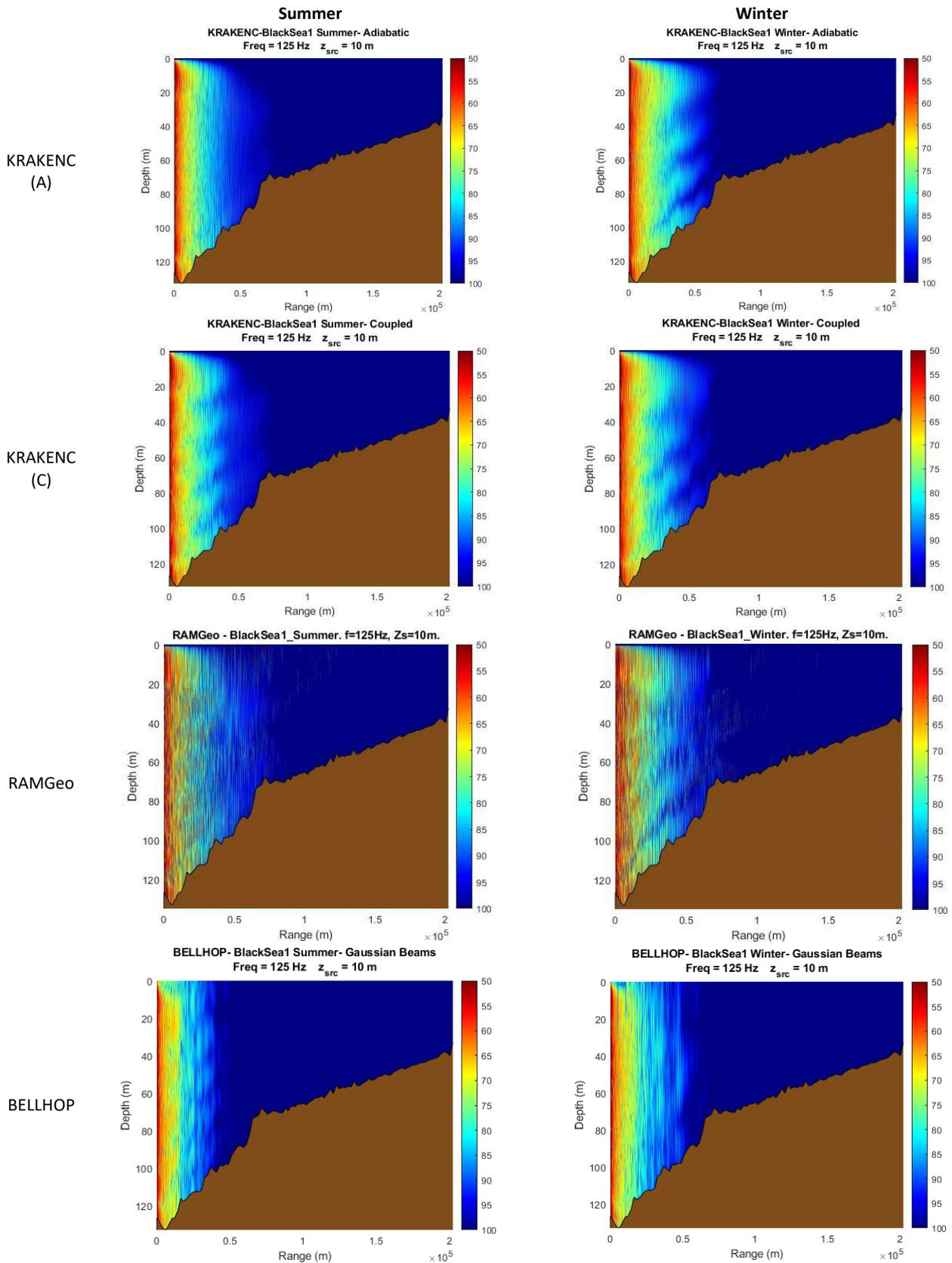
Figure 9. Acoustic propagation models outputs for summer (left column) and winter (right column) profiles and the four considered models (rows) for the 'Constanza I' test site (Area V) at 125 Hz.
