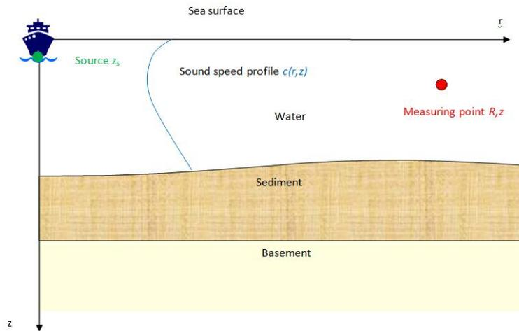
Figure 3. The vertical slice considered for the estimation of the ship noise contribution to the measuring point.
