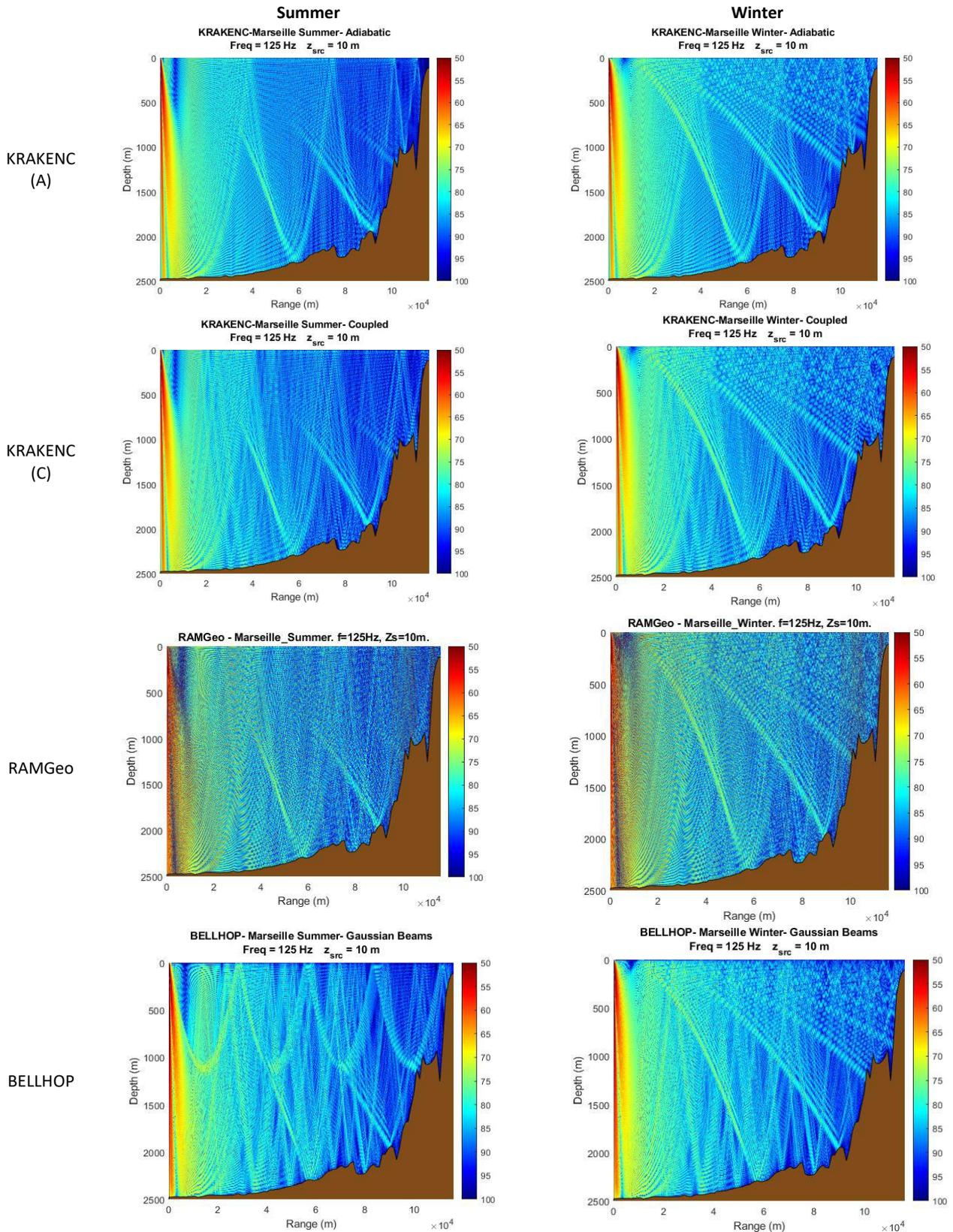
Figure 13. Acoustic propagation models outputs for summer (left column) and winter (right column) profiles and the four considered models (rows) for the Marseille test site (Area I) at 125 Hz.
