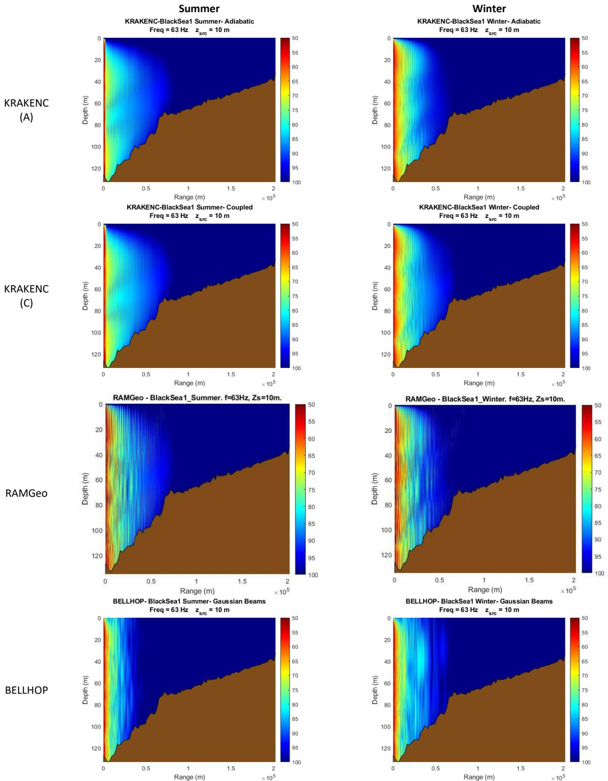
Figure 30. Acoustic propagation models outputs for summer (left column) and winter (right column) profiles and the four considered models (rows) for the 'Constanza I' test site (Area V) at 63 Hz.
