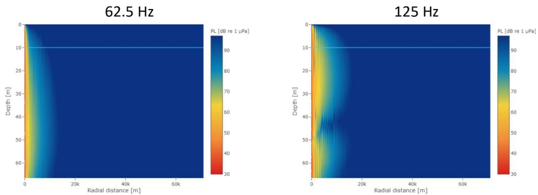
Figure 44. Propagation losses for the Black Sea I – Constanza I environment (Area V) from the URN tool using the KRAKEN model.
