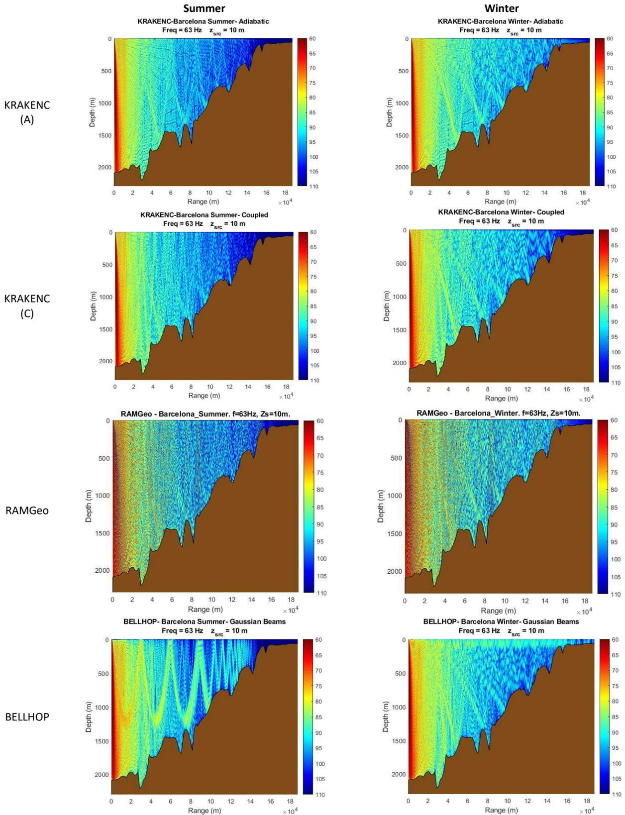
Figure 15. Acoustic propagation models outputs for summer (left column) and winter (right column) profiles and the four considered models (rows) for the Barcelona test site (Area I) at 63 Hz.
