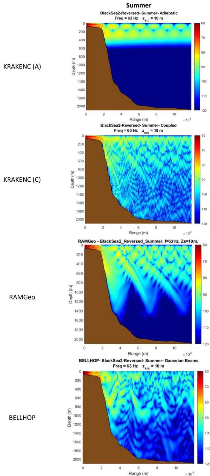
Figure 11. Acoustic propagation models outputs for summer (left column) and winter (right column) profiles and the four considered models (rows) for the ‘Constanza II RP’ test site (Area V) at 63 Hz.
